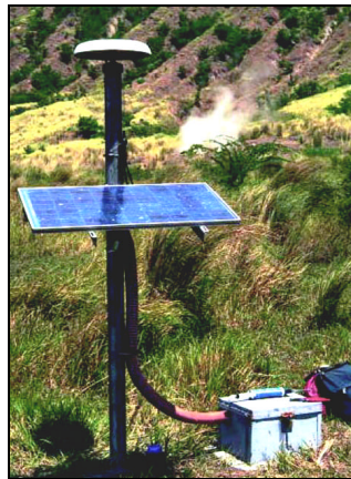
Figure 6. L1 GPS station on Taal volcano (Bartel et al. 2003)
