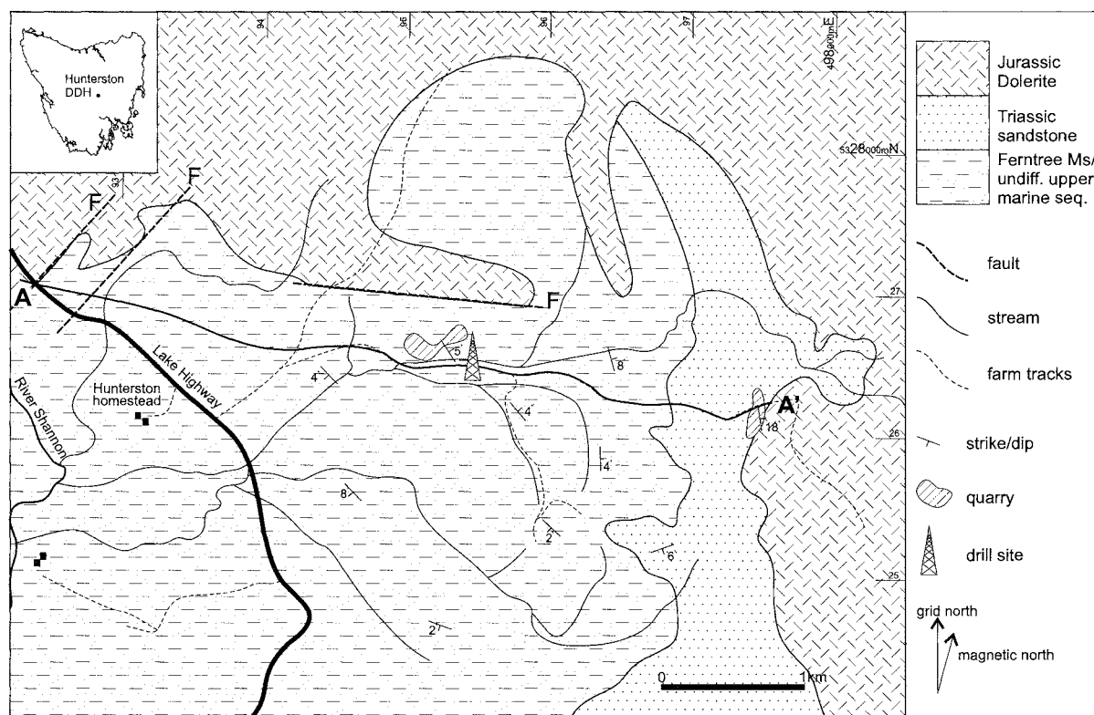
FIG. 1 — Locality map and geology in the immediate vicinity of the Hunterston DDH. A–A' approximate position of seismic line TB01-PA. See figure 7 for cross-section A–A'.
