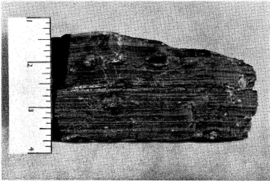
FIG. 3.—Photograph of varved mudstone from Elliott showing grading and slumping.
