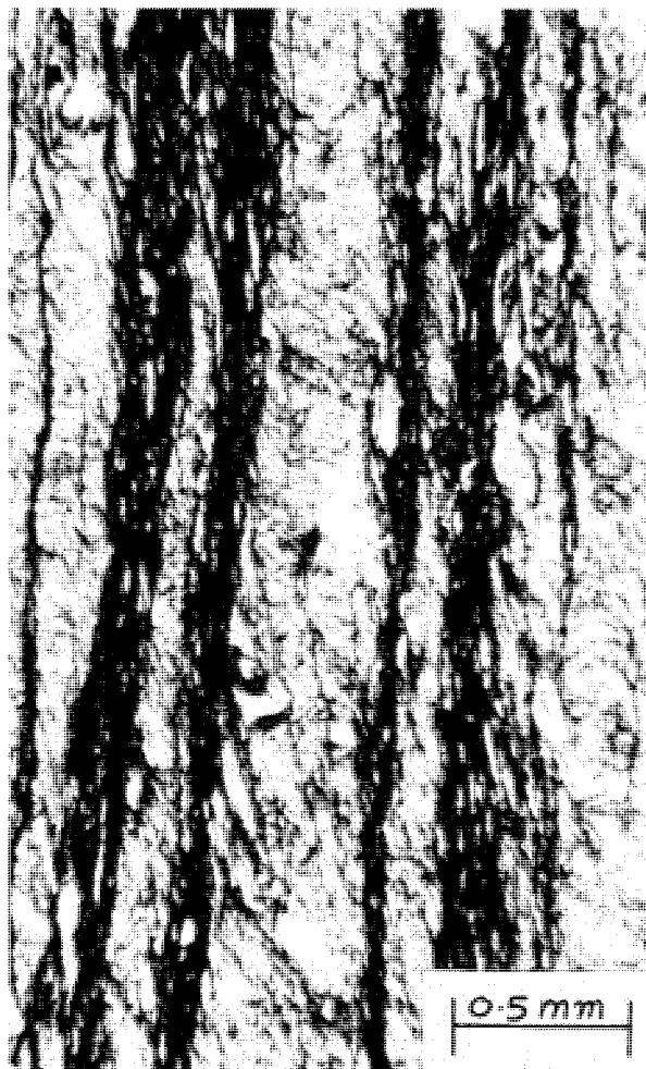
PLATE 4.-Differentiated S_3 crenulation cleavage in phyllite, with darker bands of mica growing parallel to the S_3 surface.
