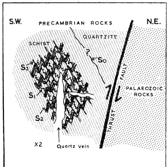
Fig. 3.—Diagrammatic section showing the relationship of the foliations in the Precambrian schists.
