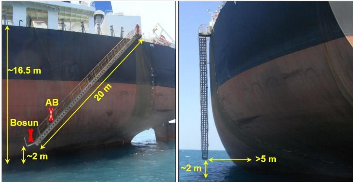
Figure 1: The accommodation ladder as rigged at the time of the accident showing distances and approximate positions of bosun and able seaman. Source: ATSB.
