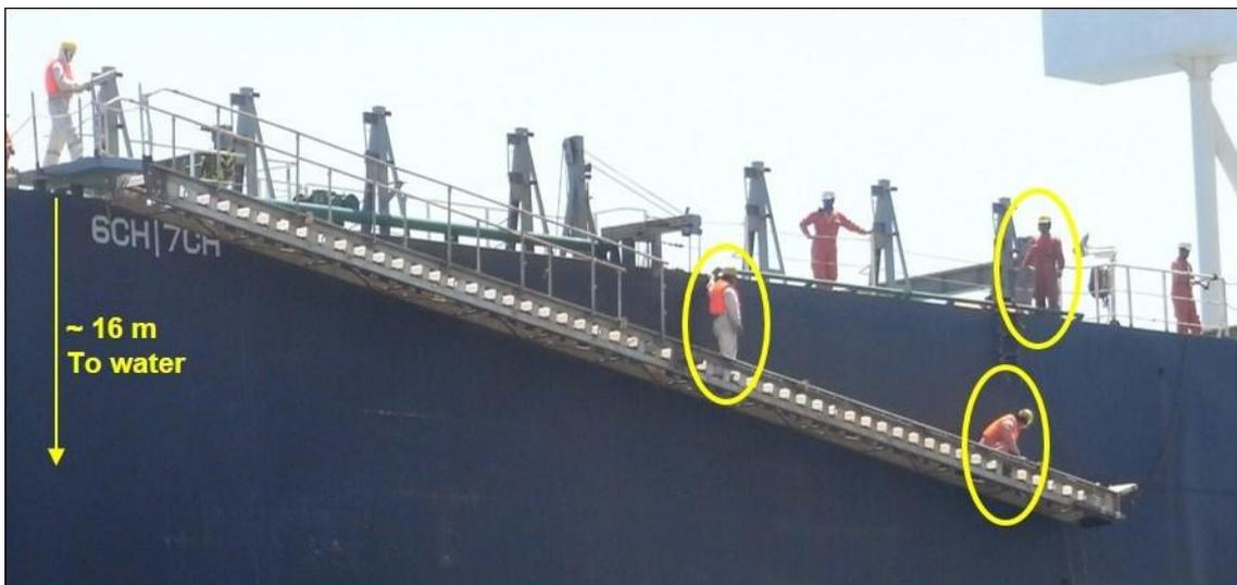
Figure 2: Crew rigging the accommodation ladder without fall protection and/or lifejacket. Source: ATSB.
