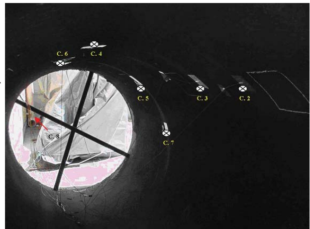
Figure 4: Pipe interior showing thermocouple locations.
