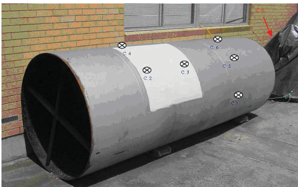
Figure 3: Pipe section in car park. Thermocouple locations indicated.
