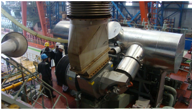
Figure 6. Turbocharger for a large two stroke engine at test bed in QMD, Qungdao, China.
