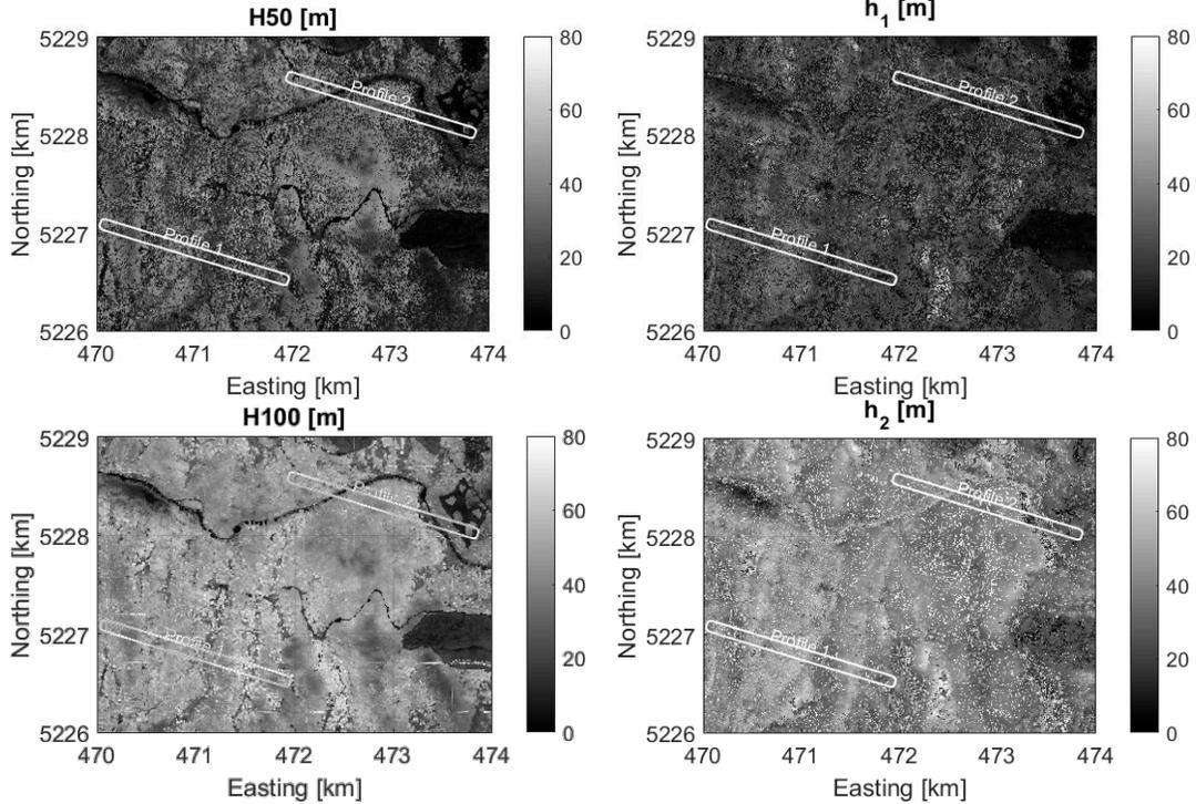
Figure 1: Comparison between H50 and H100 measured with airborne lidar scanning and  $h_1$  and  $h_2$  obtained from 3LM inversion of multi-temporal TanDEM-X data. All images are in UTM55N coordinates.
