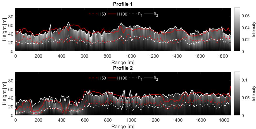
Figure 2: Examples showing three backscatter profiles along the transects shown in Figure 1, together with H50 and H100 from ALS and  $h_1$  and  $h_2$  from 3LM inversion. The profile locations are outlined in Figure 1 and the range is measured from the south-east end.
