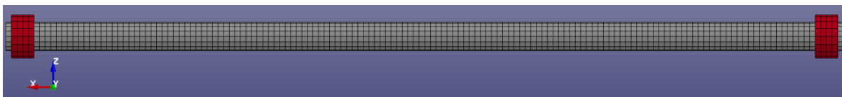
Figure A1-5 Configuration 1 – 4 collars [400 kg] at each end
