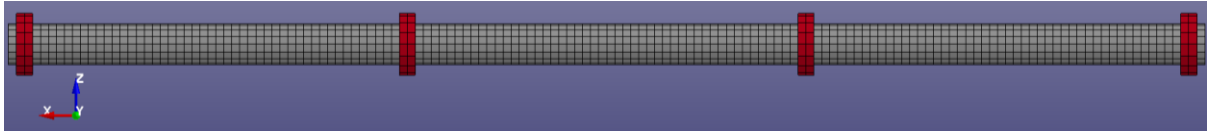
Figure A1-8 Configuration 4 – 2 collars [200 kg] at each end & 2 collars [200 kg] at each peak
