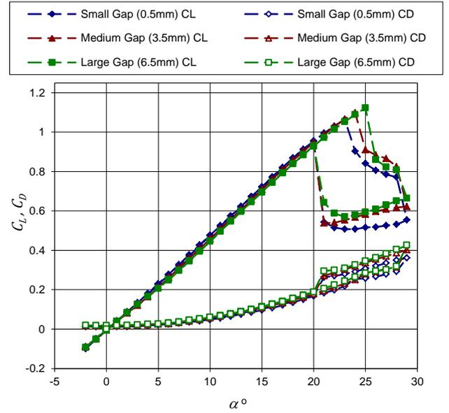
Figure 6. Lift and drag coefficients for the control surface with gap size for a  $Re_{root}$  of  $1.25 \times 10^6$  with an injection ratio of  $C_{p,inj} = -0.565$ . The filled symbols represent the lift coefficient,  $C_L$  and the hollow symbols show the drag coefficient,  $C_D$ .
