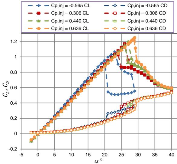
Figure 8. Lift and drag coefficients for the control surface with boundary layer thickness for a  $Re_{root}$  of  $1.25 \times 10^6$  with a small gap (0.5 mm). The filled symbols represent the lift coefficient,  $C_L$  and the hollow symbols show the drag coefficient,  $C_D$ .
