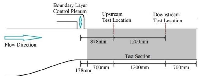
Figure 3. Schematic showing location of boundary layer control plenum and test positions in the AMC cavitation tunnel.
