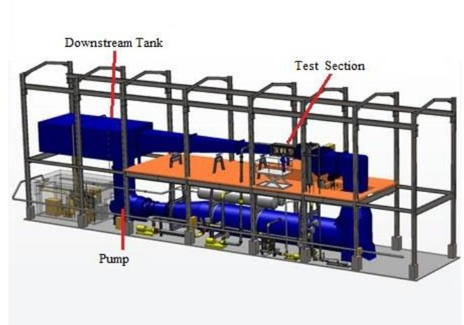
Figure 2. CAD image of the AMC cavitation tunnel<sup>[1]</sup>.
