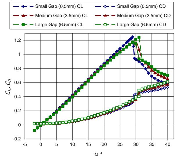
Figure 7. Lift and drag coefficients for the control surface with gap size for a  $Re_{root}$  of  $1.25 \times 10^6$  with an injection ratio of  $C_{p,inj} = 0.440$ . The filled symbols represent the lift coefficient,  $C_L$  and the hollow symbols show the drag coefficient,  $C_D$ .
