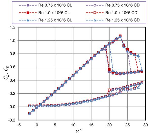
Figure 9. Lift and drag coefficients for the control surface with a gap size of 0.5mm and  $C_{p,inj} = -0.565$  for a  $Re_{root}$  between  $0.5 \times 10^6$  and  $1.25 \times 10^6$ . The filled symbols represent the lift coefficient,  $C_L$ , and the hollow symbols show the drag coefficient,  $C_D$ .
