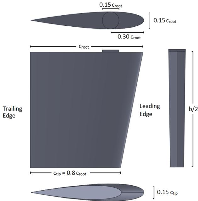
Figure 1. Canonical control surface design: NACA0015 section, taper ratio 0.8, no trailing edge sweep, and semispan equal to root chord.
