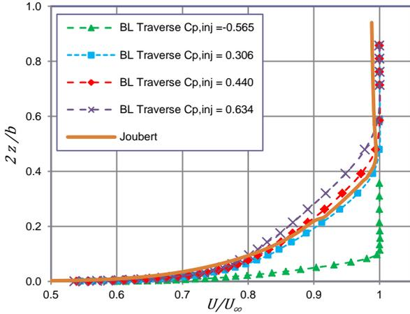
Figure 4. Measured boundary layer profiles at  $Re_{root} = 1.0 \times 10^6$  and nominal boundary layer profiles in vicinity of aft control surface for the Joubert hullform<sup>[4][5]</sup>.
