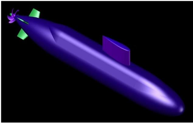
Figure 5. Fully appended Joubert 'generic' diesel submarine hullform.
