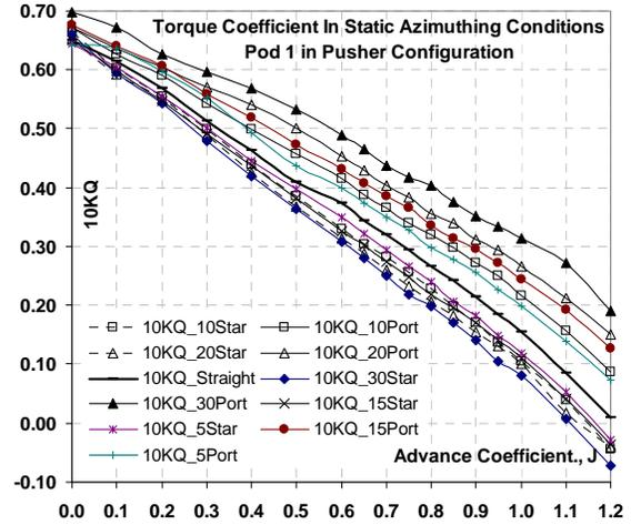
Figure 16. Propeller torque coefficient for Pod 1 unit at different azimuth conditions.
