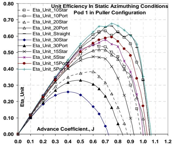
Figure 12. Unit efficiency plots for Pod 1 at different azimuth conditions.
