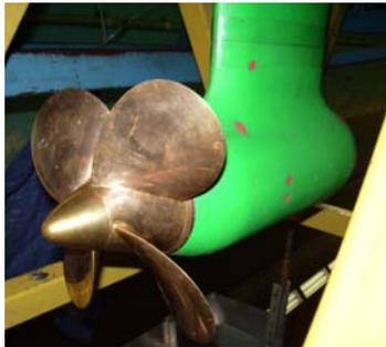
(e) propeller and the pod enclosing the pod dynamometer
