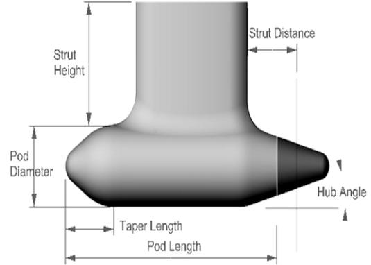
Figure 1. Geometric parameters used to define pod-strut geometry.
