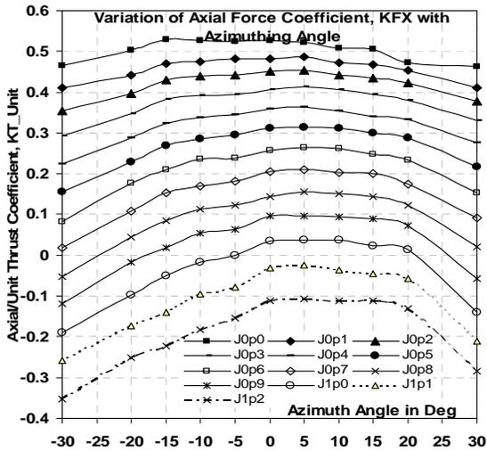
Figure 20(a). Unit thrust / Longitudinal force coefficient
