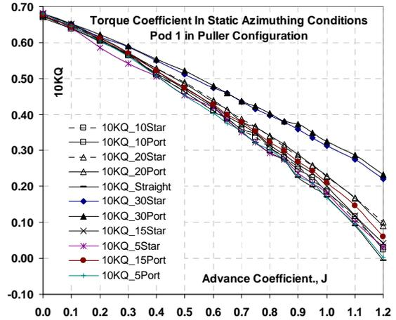
Figure 11. Propeller torque coefficient for Pod 1 unit at different azimuth condition.
