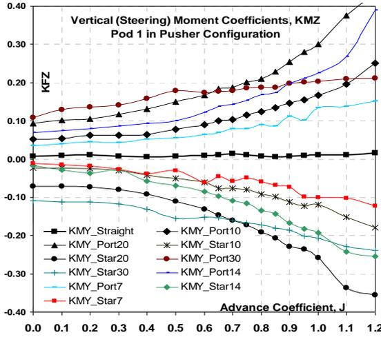
Figure 19. Vertical (steering) moment coefficient plots for Pod 1 at different azimuth conditions
