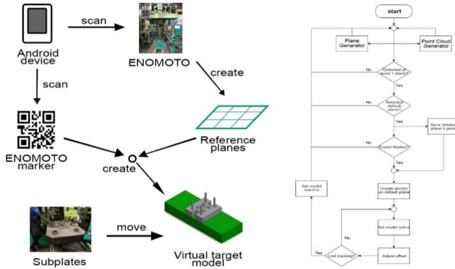
**Figure 3.** System overview (a) system diagram (b) program flowchart
