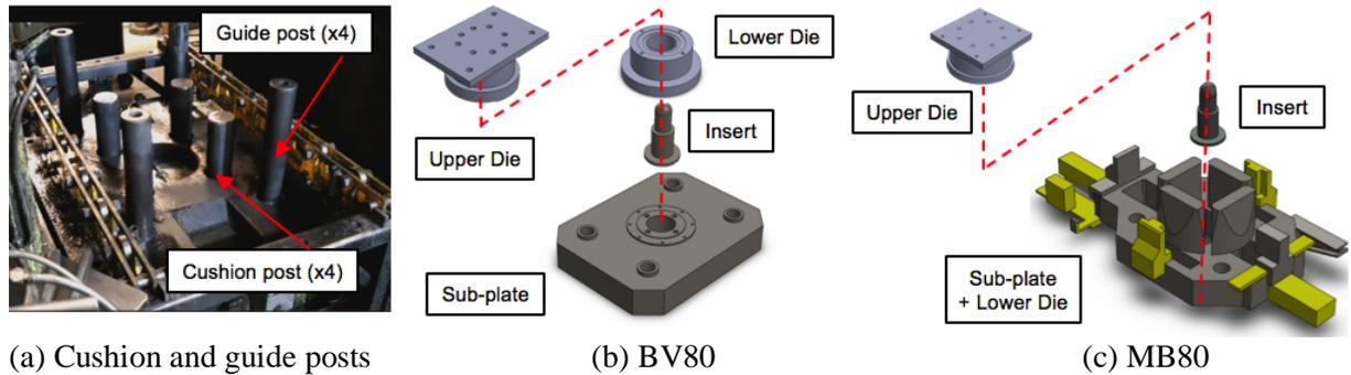
**Figure 1.** Components in the machine and dies set [5]
