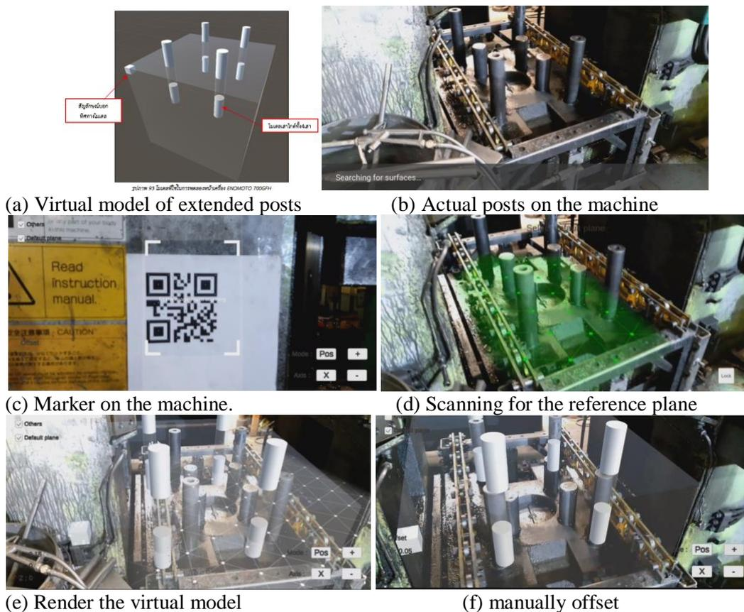
**Figure 4.** Experiment on shop floor
