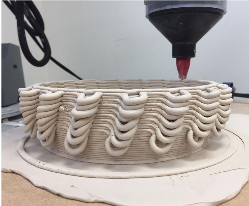
*Figure 4 Ceramic 3D printing of the Hybrid material vessels #2, clay loops can be seen “drooping” as it is pushed out of the Potterbox printer, due the loops being unsupported and the forces of gravity.*
