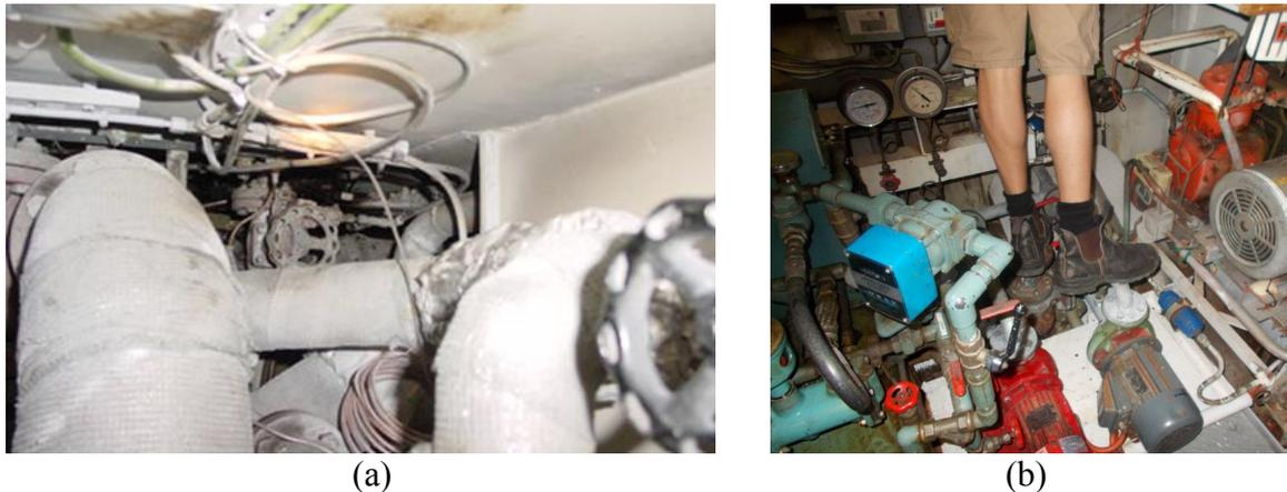
**Figure 2** An activity of students checking accessibility/operability of valves inside the engine room. (a) Regularly used valve position leading to awkward work posture; (b) Operators' position to reach a valve.
