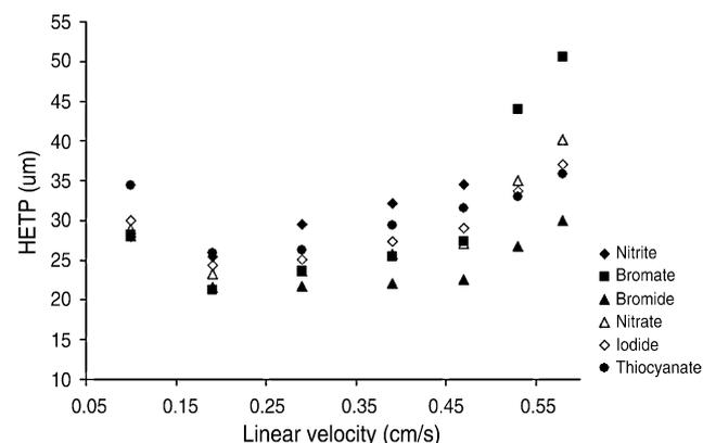
Fig. 5. van Deemter plot for anions on the 10 cm lysine modified silica monolith. Eluent = 20 mM phosphate eluent (pH 3.0).
