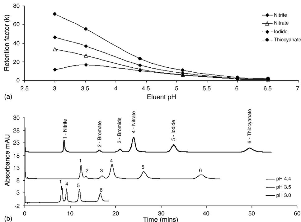
Fig. 3. Effect of eluent pH on anion capacity. (a) Eluent = 1 mM phosphate buffer; flow rate = 1 mL/min; detection = 214 nm. (b) Eluent = 2 mM phosphate buffer; flow rate = 2 mL/min; detection = 214 nm.
