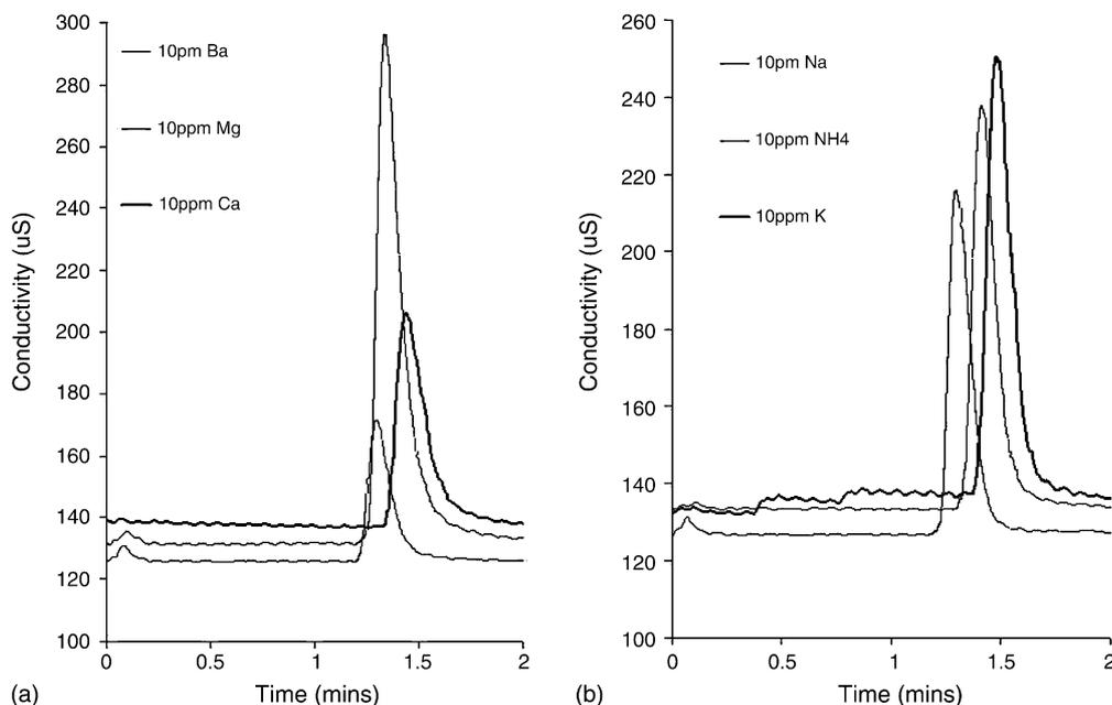
Fig. 1. Overlays of chromatograms for (a) alkali and (b) alkaline earth metal ion standards obtained on the lysine modified monolith. Conditions: eluent = 3 mM HNO<sub>3</sub>; flow rate = 1 mL/min; detection = suppressed conductivity.
