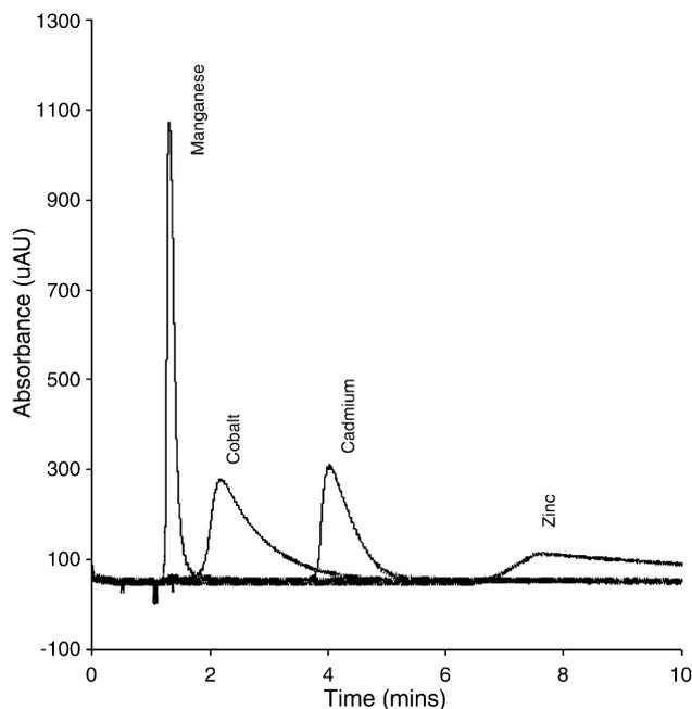
Fig. 2. Overlay of Mn(II), Co(II), Cd(II) and Zn(II) chromatograms obtained on the lysine modified monolith. Conditions: eluent = 3 mM KCl, pH 4.5; flow rate = 2 mL/min; detection = post-column reaction with PAR, absorbance at 495 nm.
