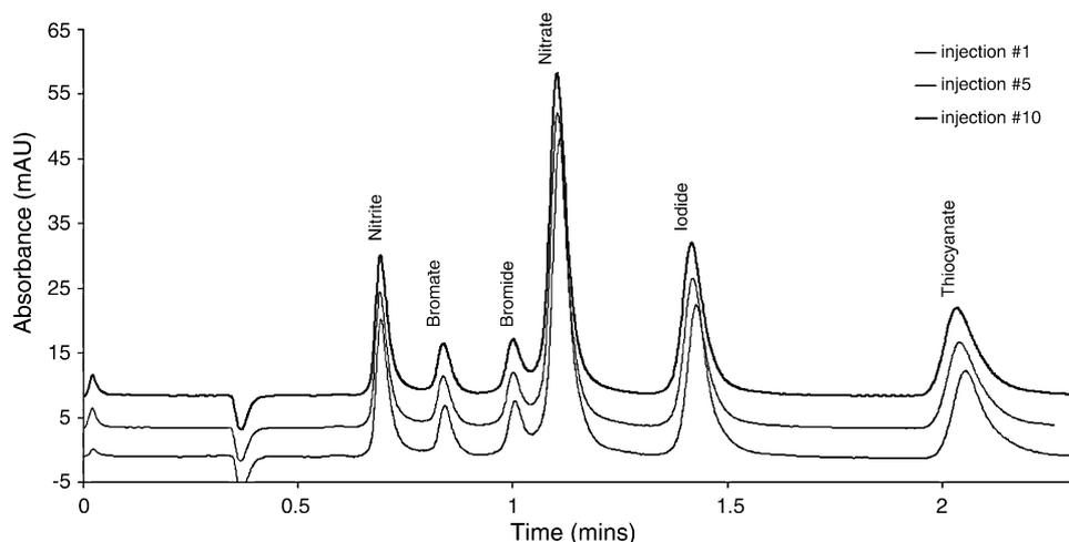
Fig. 8. Overlaid chromatograms from precision study carried out using the lysine modified monolith. Eluent = same as Fig. 6. Flow rate = 4.0 mL/min.
