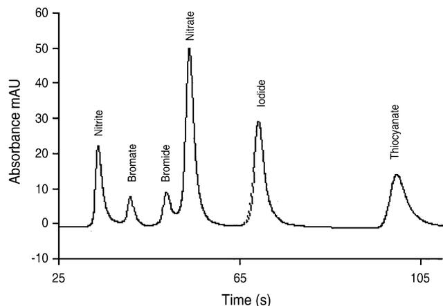
Fig. 6. Separation of 6 anions in 105 s using the lysine modified monolith. Eluent = 50 mM phosphate (pH 3.0); flow rate = 4.9 mL/min.
