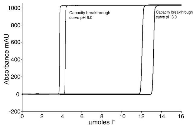
Fig. 4. Overlaid breakthrough curves performed on the lysine monolith using 1 mM KI at pH 3.0 and 6.0, delivered at 1 mL/min.
