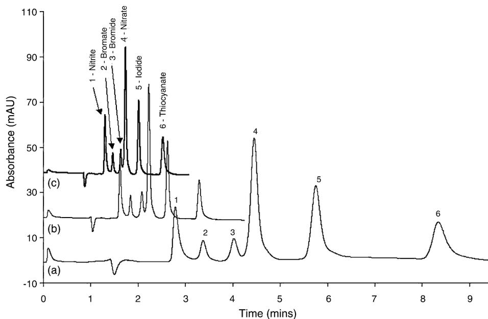
Fig. 7. Overlaid chromatograms obtained using the lysine modified monolith under: (a) isofluentic conditions at 1 mL/min; (b) flow gradient conditions from 1 to 4.9 mL/min over  $t = 0$ –4 min; (c) flow gradient conditions from 1 to 4.9 mL/min over  $t = 0$ –2 min. Eluent = same as Fig. 6.
